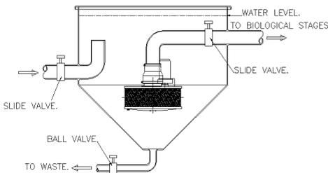
the unit is located as near to mid-height in the vortex as possible. This although not being critical gives better performance of the unit. N.B. What is important is to have the inlet pipe vertical and level with half way up the screen of the unit as shown above. If 'The Answer' is fitted upside down, the inlet pipe must be brought up vertically, but NOT too close to water surface level as this reduces pressure in the pipe for line purges (150mm below
