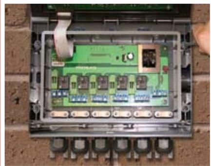
**3** To connect the power cable, you'll need 13mm diameter armoured cable, connected to a mains power supply. Thread the power cable with exposed ends through the grey connector and into the switch box. Unscrew the necessary cable, pin and connector clamps to allow you to wire in the earth, live and neutral connections.
