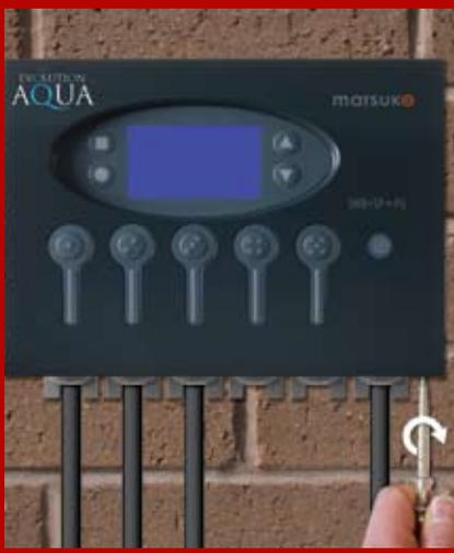
**6** Turn the switch box on at the mains. Once activated, the power light will illuminate and the screen will display a welcome message, followed by the main menu screen.
