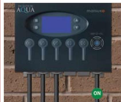
**7** On the SwitchMaster Pro model, every device can be programmed to turn on and off at set times at your convenience (see page 64).
