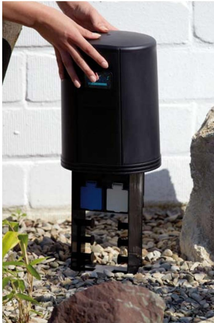
against moisture. This is referred to as the Ingress Protection (IP) rating. Ratings read 'IP', followed by two numbers. The first indicates the level of protection offered against solids, and the second the protection against liquids. If either of the numbers is represented with an 'X', this means that the item hasn't been tested.
