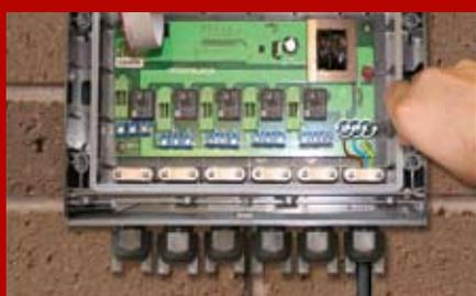
**4** Wire in every device you need to connect up, as instructed by the installation manual.
