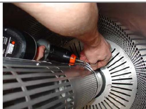
14. Connect the new back wash air tube from the Eazy to the top air valve
