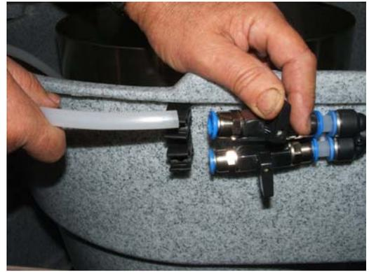
15. Connect the existing air-ring air tube to the lower valve on the "Y" connector.
