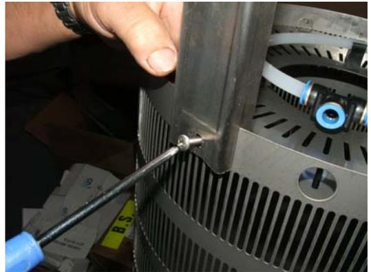
9. Connect the new backwash air tube to the "Eazy" aeration ring
