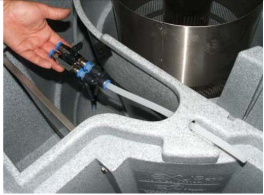
7. Attach the Y Air valve assembly by screwing the self tapping screw through the inner chamber into the center of the Y piece
