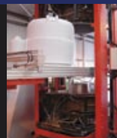
STAGE FIVE The Nexus 300 is now around 60°C and is transported to the slide for final assembly
