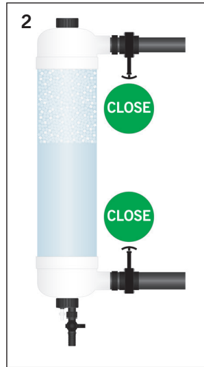
STEP 2 Close both slide valves
