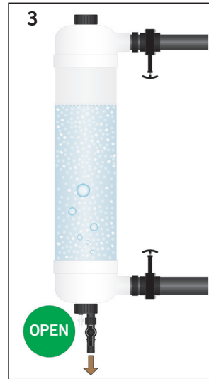
STEP 3 Open waste valve tap
